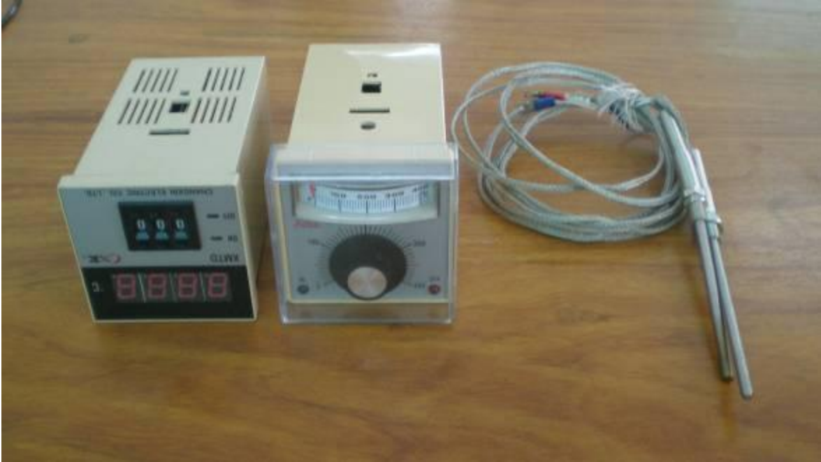
A view of thermocouple, temperature control, and indicator.
