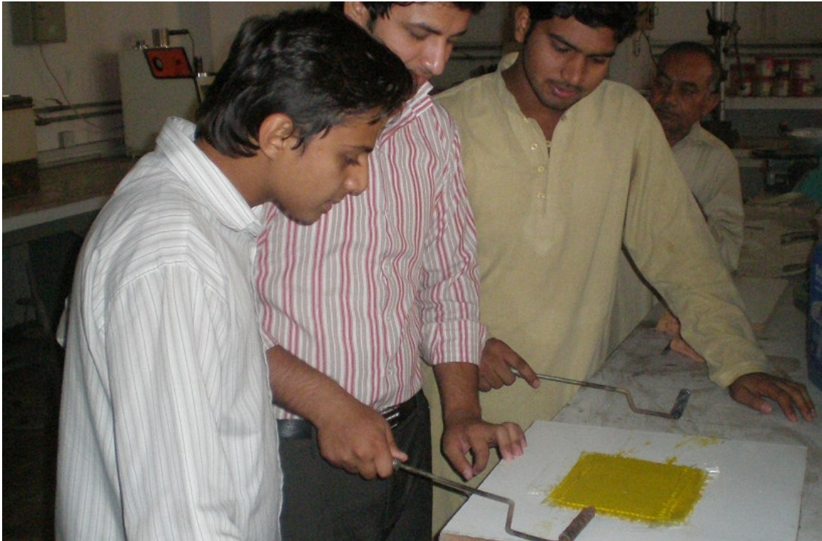
Making a Polymer Matrix Composite using Polyester & E-Glass Fibers
