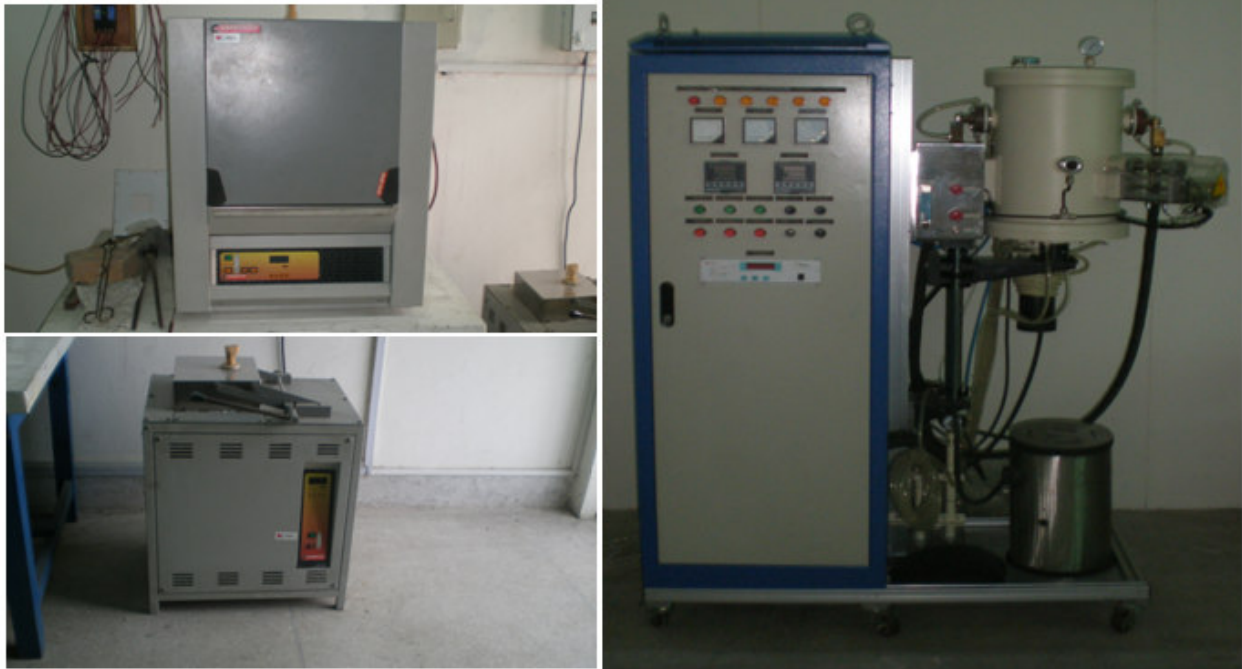
Carbilite heat treatment furnaces and a high vacuum sintering furnace
