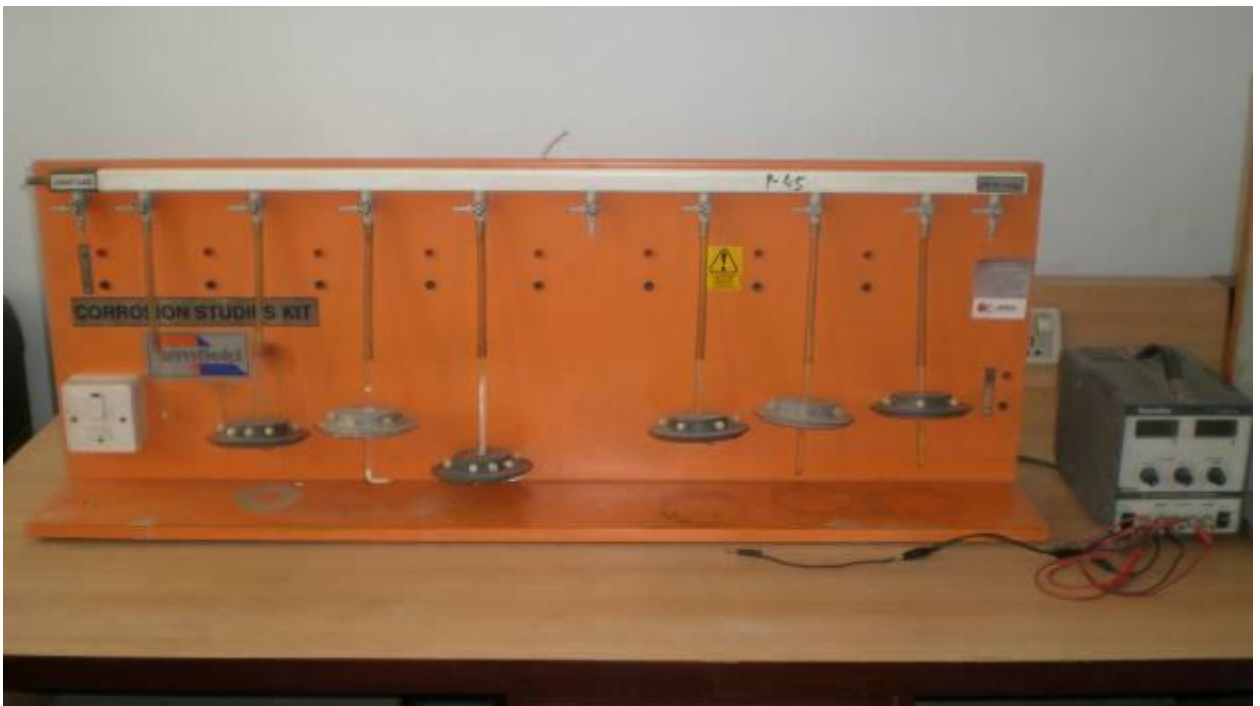
Corrosion kit to observe the corrosion behavior of metals.
