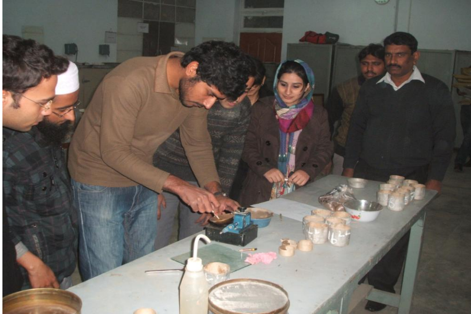
Performing Atterberg Limits Test
